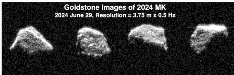
Selected delay-Doppler radar images of 2024 MK obtained on June 29 when the asteroid was at about one lunar distance and approaching Earth. Resolution is 3.75 m x 0.5 Hz. Each panel shows a weighted sum of data that span about 20 seconds. DSS-14 transmitted and DSS-13 received.
